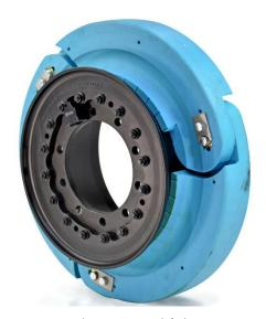
**Static 100km**: a 3-segment system designed and manufactured to cover 100 km on road (3km at escape speed up to 90km/h, 22km at 50km/h and 75km at 25km/h) or 60 km off road at 30 km/h in run flat mode.
